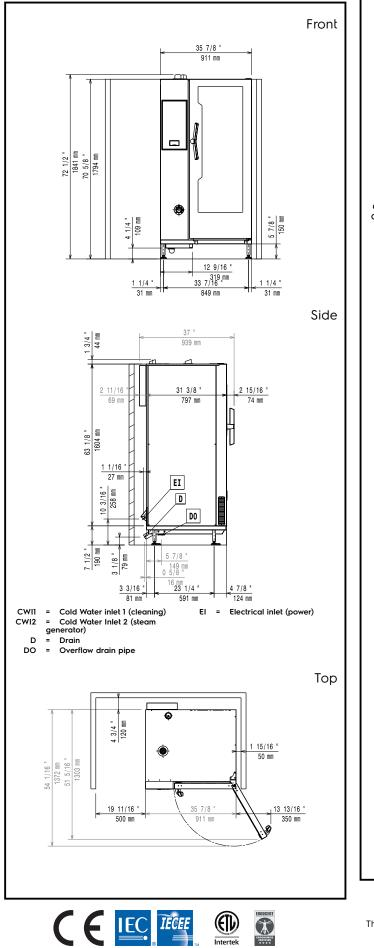
Distances CWI1 1 15/16 50 mm CW12 4 3/4 ' 120 nn > 15/16 EI DO <u>4 7/16</u> 10 1/16 113 nn CWII Cold Water inlet 1 (cleaning) EI = Electrical inlet (power) = = Cold Water Inlet 2 (steam generator) CWI2 D Drain = = DO Overflow drain pipe
